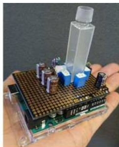
Fig. 2 A homemade palmtop spectrophotometer.
